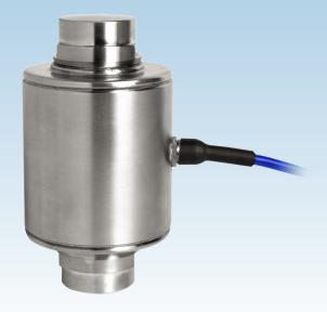
This stainless steel self-centering rocker column load cell is fully welded and hermetically sealed, with protection to IP68/IP69K. It is an ideal solution for weighbridges/truck scales thanks to its approval to OIML C3 (3000 divisions), as well as in-built lightning surge arrestors and a tough, durable polyurethane cable. Anti-rotation is achieved by means of 2 flat faces on either side of the load cell base, with corresponding flat faces in the lower mounting cup.
