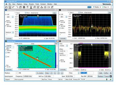
Once captured into memory, SignalVu-PC provides detailed analysis in multiple domains. The spectrogram display (bottom left panel) shows the frequency of an LFM pulse changing over time. By selecting the point in time in the spectrogram during the On time of the pulse, the chirp behavior can be seen as it sweeps from low to high (upper right panel).
