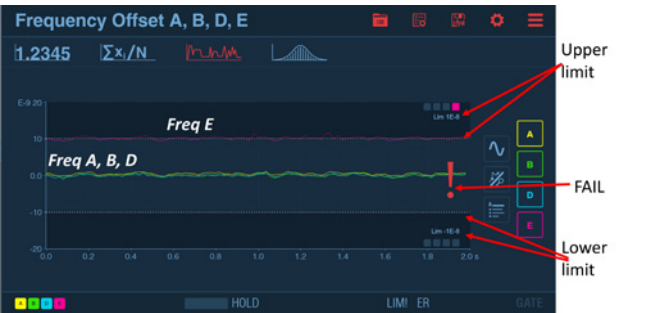
The time-line view reveals drift during the calibration
