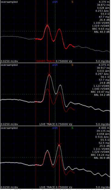
Figure 1: TDR waveform of a standard 50 Ohm Male-Male barrel connector (2.5 cm/div). The first screenshot shows both connectors properly tightened with an associated saved trace (red). Subsequent screenshots show the first connector incompletely tightened with a ~6 dB higher return loss than expected, then the second connector incompletely tightened with ~4 dB higher return loss than expected.
