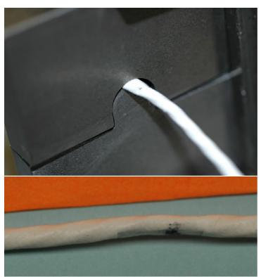
Figure 3: Non-destructive clamp fault, causing deformation of the shield and underlying twisted-pair but no significant permanent damage following its removal. There would likely be no significant impairment of system performance.
