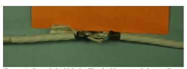
Figure 4: Partial shield fault. The shield remained electrically contiguous with no significant DC resistance. The underlying twisted pair is undamaged.
