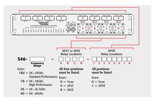
**Multipole Relay Locations A–D:** Enter a "4" for an SP4T relay or a "6" for SP6T relay in the required location. Enter a "0" in unused multi-pole locations. There must be digits in all four positions.
