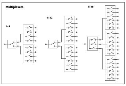
$\textbf{MAXIMUM CONFIGURATION:} \ (8) - Unterminated \ SPDT \ relays. \ (4) - Unterminated \ multi-pole \ relays \ (SP4T, SP6T).$
