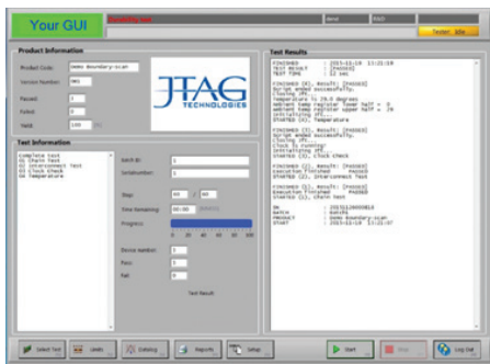
Figure 3: Example of a LabVIEW-based GUI combining PIP/LV functions with functions for other instruments
