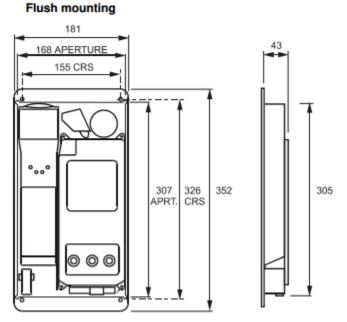
Titan telephones supplied for flush mounting have a slightly different faceplate to those supplied with a rear enclosure – in particular the fixing holes are in different positions and there are no corner cut-outs (for door hinges). These models are described as «Titan fp» and the supplied mounting kit contain round-headed scews and no glands.
