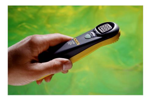
**Fluke CO-220** Fluke CO-220 Carbon Monoxide Meter
