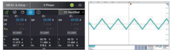
PU mode: freely set peak current for captured or user-defined waveforms
