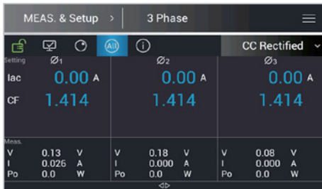
CC Rectified Mode (Three Phase)
