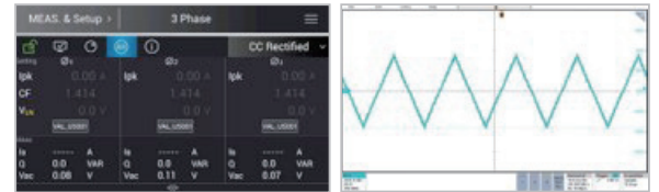
VAL mode: full replication of captured or user-defined waveforms
