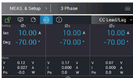
CC Lead/Lag Mode (Three-Phase)
