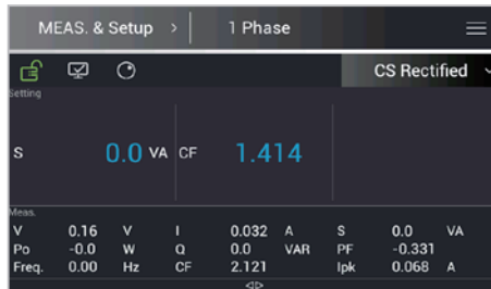
CS Rectified Mode (Single Phase)
